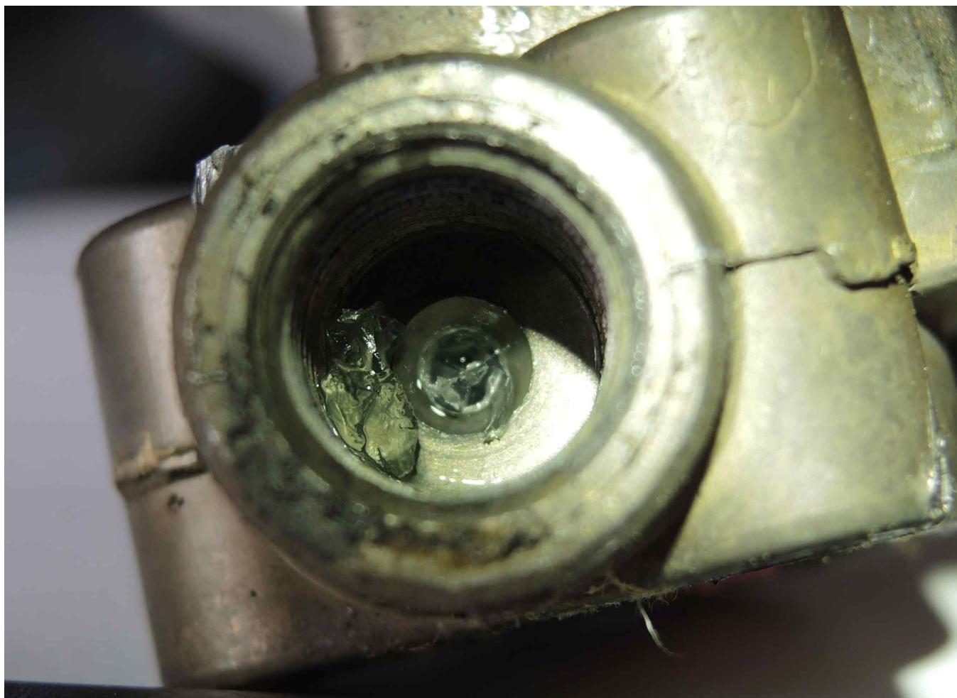
Photo 1 - Fuel Flow Transducer Inlet Port
