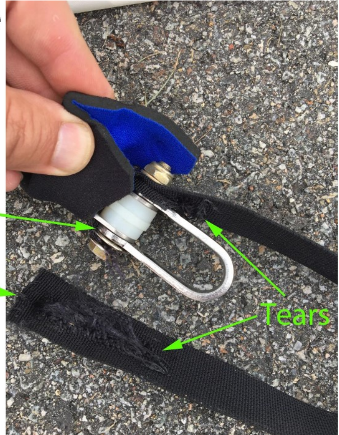
Figure 1. Cable shackle and pull handle. Note tears in nylon webbing.
