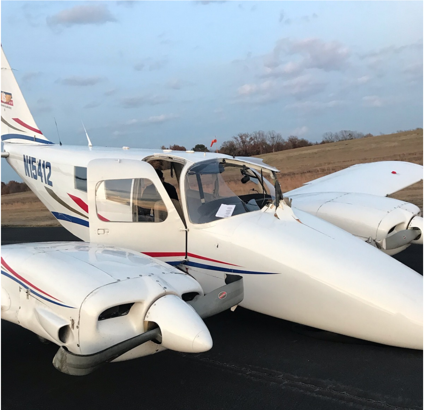
Figure 1 – Airplane with nose gear strut through the fuselage and windscreen
