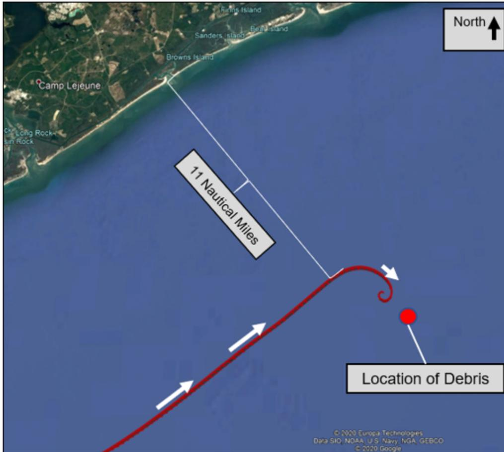
Figure 1: The airplane's final 3-minutes of flight track data (red line) and location of debris (white arrows show the airplane's direction of travel).
