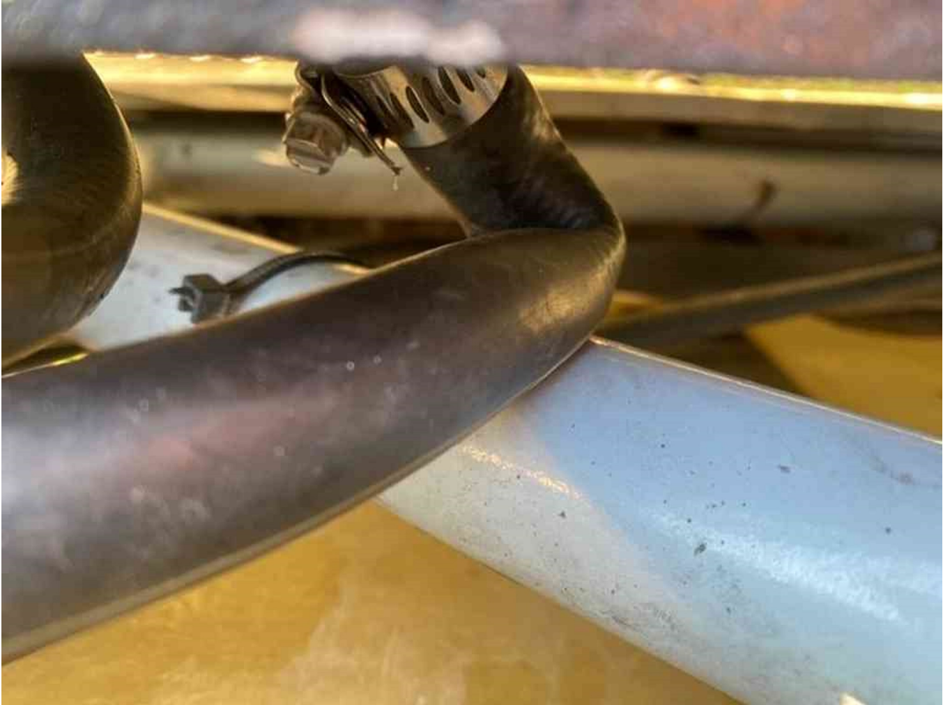
Figure 1. Creased Fuel Vent Right Wing
